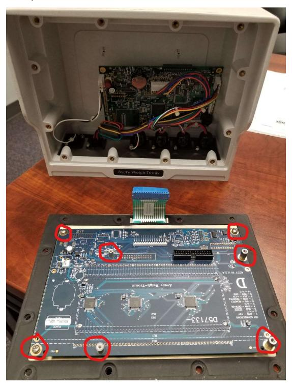
Connect the ribbon cable from the overlay and backer assembly to the display board and close the latch:
