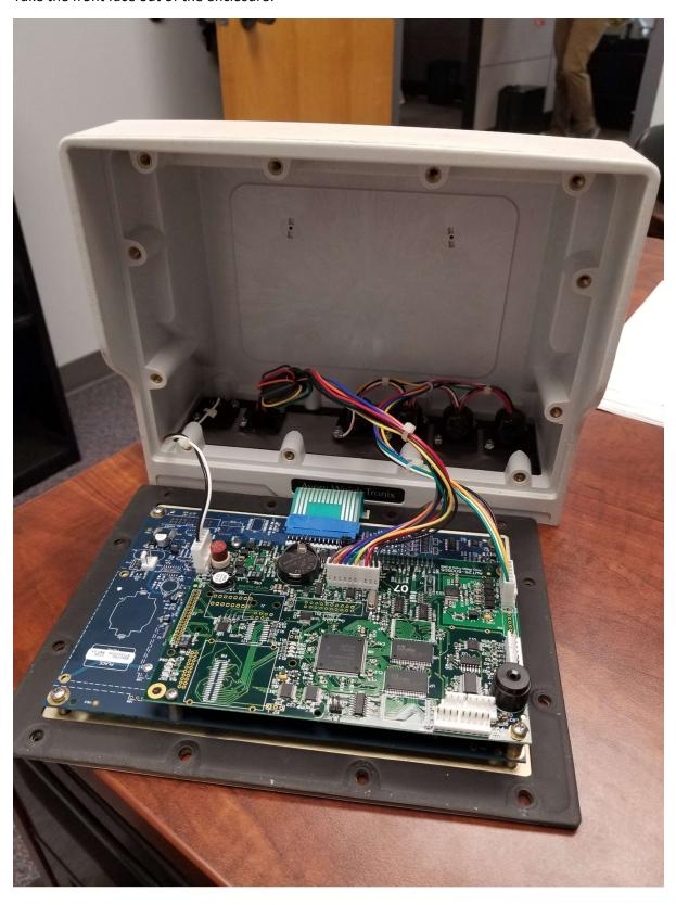
Remove the screws that hold the main board to the display board (4) and remove the main board from the display board. After the screws are removed there is a multi-pin connector that will still be connecting the main board to the display board. Wiggle this connection gently while pulling up, and this connector will become unseated:
