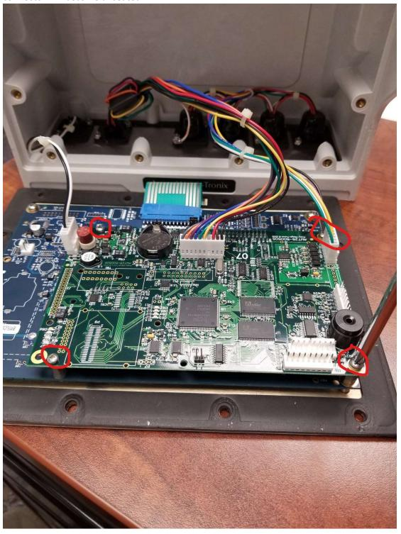
Remove the ribbon cable from the display board. Lift up the latch that adds tension to the pins then gently wiggle the connector free of the pins:
